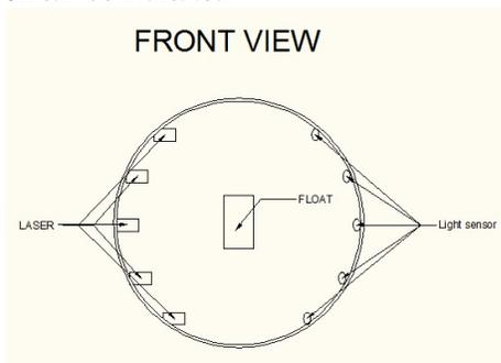
Figure 8: Front inside view of conservator showing the arrangement of laser and light sensor.
