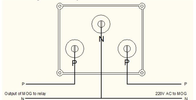
Figure 6: Connection diagram of MOG
