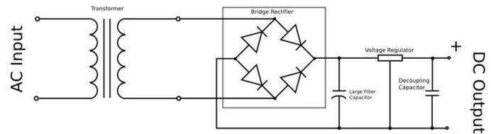
Figure 2: Linear power supply circuit
