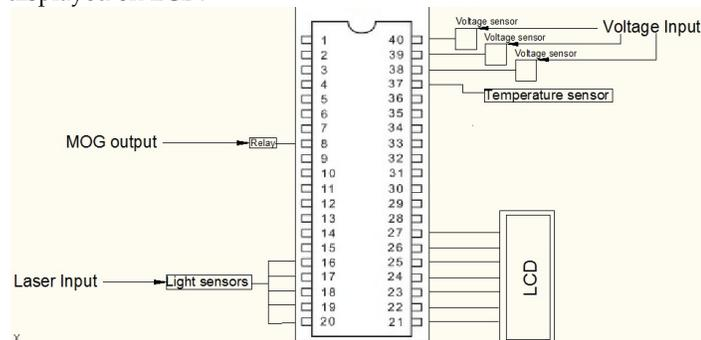
Figure 9: Connection diagram of system
