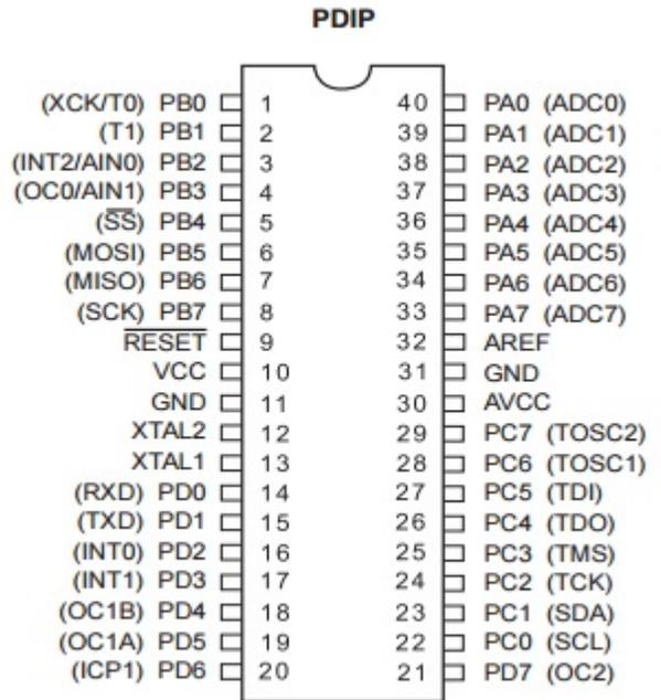
Figure 5: Atmel AVR pin outs
