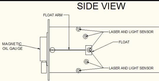
Figure 7: Side view of conservator showing the arrangement of laser and light sensor
