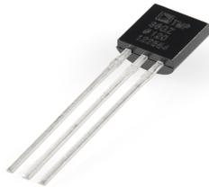
Figure 4: Temperature sensor TMP36
