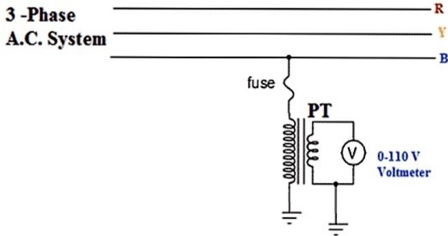
Figure 3: Arrangement of potential transformer
